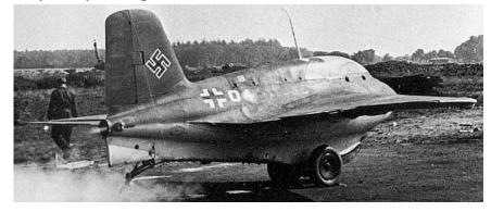
takeoffs and dead stick landings were white knuckle affairs due to the lack of landing gear. 80% of Me-163 accidents happened on takeoff or landing. Even its speed became a drawback. A *Komet* pilot only had 3 seconds to fire on the slow-moving bomber before breaking away to avoid a collision.
