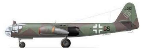
Arado's clean and elegant design, powered by 2 Junkers turbojets like the Me-262, would be so fast that no defensive armament was deemed necessary. Like all fantasies, however, reality has a way of intruding. The Junkers engines were behind schedule and proved to be unreliable, and the clean design of the "Blitz" was partly due to having no landing gear. Taking off with a jettisonable dolly and landing on =------>
