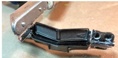
Dual headlight lights were cut out.
