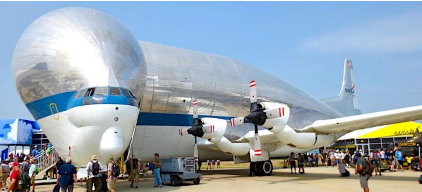
Boeing's display area included two of the biggest aircraft in its inventory. NASA's Super Guppy was designed to carry large loads from the space program and is the last operational Boeing 377 turboprop in existence.
