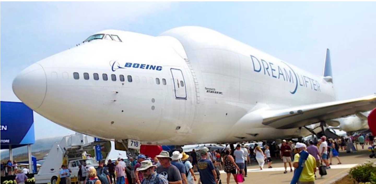
The Boeing DreamLifter is a heavily modified 747 that carries equipment and parts around the world that are too large for normal shipping methods.
